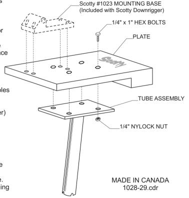
NOTE: <u>Downriggers must face aft while fishing</u>. If downriggers faced outwards, the twisting force will damage the rodholders
